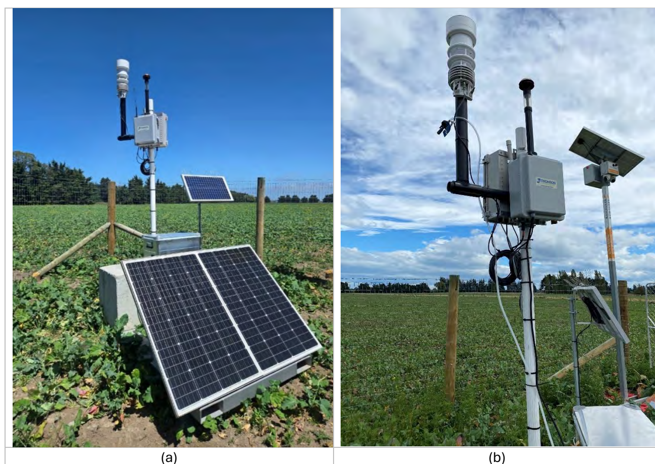
Figure 3.2: Monitoring installation at the Templeton monitoring location: (a) monitoring setup in November 2025, photographed by PortHill; and (b) same monitor on 13 February 2026, showing the respirable sampling cyclone attached to the support arm, photographed by Fulton Hogan.
