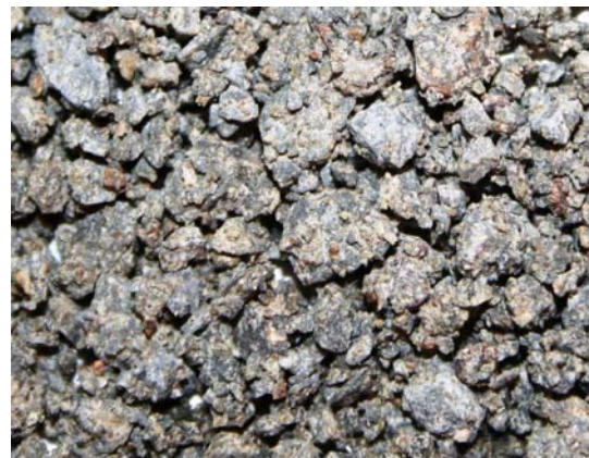
Figure 5. PAP aggregate coated with dust and fine particles.
